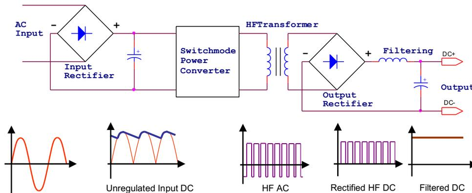
Fig. 2: Typical isolated high frequency battery charger
