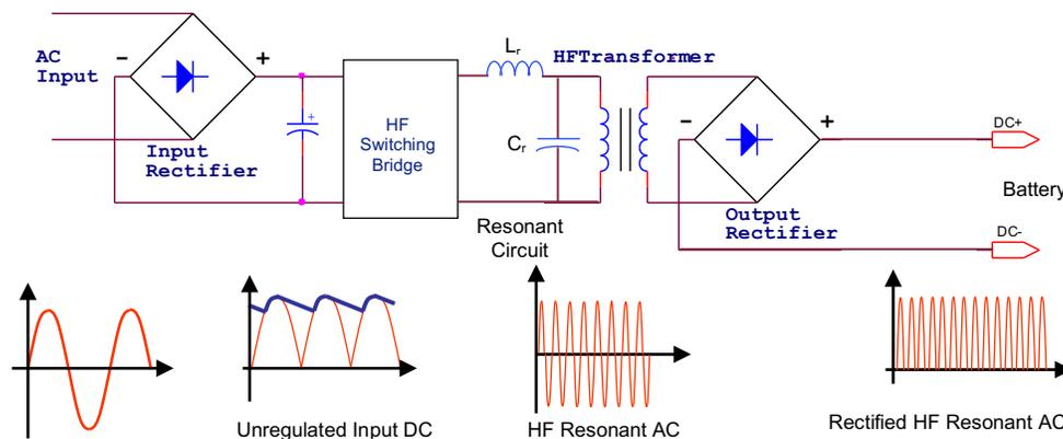
Fig. 3: High frequency, high AC ripple resonant battery charger
