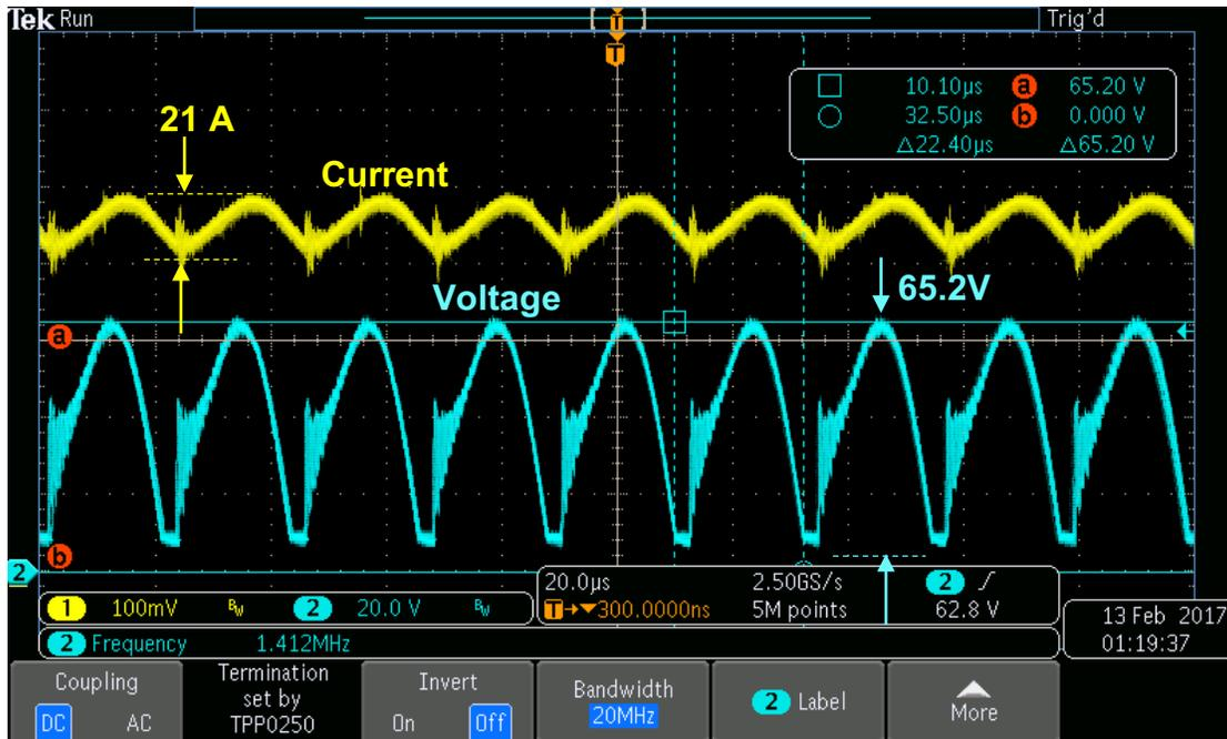
Fig. 4: High frequency output voltage of the LifePlus, PowerTech, and Enforcer chargers
